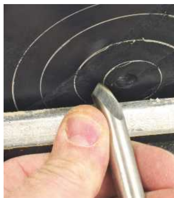
▲ Pic.9 There are many tricks to help you make the first cut. A good one is to use your thumb to fix the tool against the toolrest. As the tool is advanced forward, it can't move sideways
